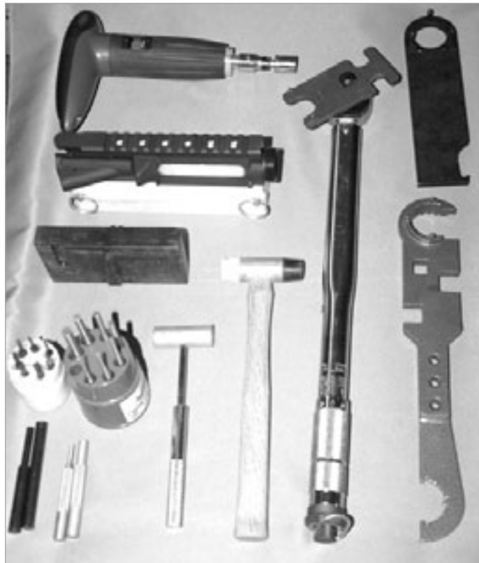
Some of the basic tools needed for AR assembly include (clockwise from L to R) a good torque wrench, barrel nut wrenches, non-marring hammers, punches and lower and upper receiver blocks. Photo courtesy of Rifleman Consulting LLC.
